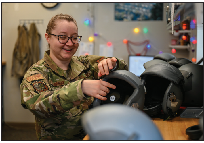
Staff Sgt. Gabrielle Saidak, 445th OSS aircrew flight equipment technician, inspects HGU-55/p helmets for defects or other damages at Wright-Patterson Air Force Base, March 23, 2025.
